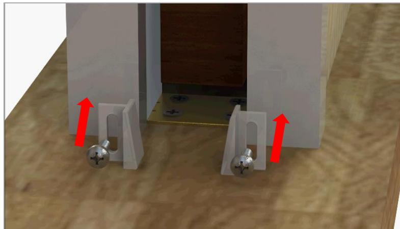
Apply desired wall material. Wall material is brought clear to edge of opening.
