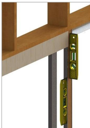
Ensure studs are straight (on the front and on the side). To double check if everything is straight the floor plate must be located in the middle of the chalk lines.
