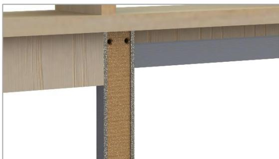
Place a split stud on the track and butt it up to the head, pre-drill and countersink holes for fixing screws, in the wood header NOT THE TRACK. Repeat the step for all the split studs.
