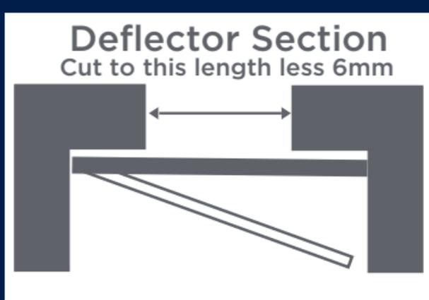
2. Using a fine toothed hacksaw, cut the aluminium 6mm shorter to allow for protective weather deflecting end caps.
