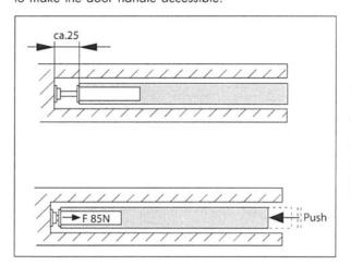
In the wall pocket behind the opened door you only need a space of 25 mm for the buffer. At the end of the piston rod is a magnet that keeps the door safely in the opened position. If the door or frame is not made from metal, you need a small metal plate (e.g. a washer) as a counter part.
